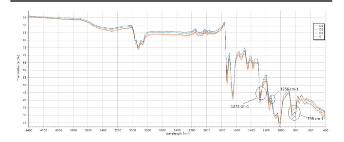
Figure 6. ATR-FTIR result of dicyandiamide applied leathers
