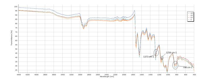
Figure 4. ATR-FTIR result of urea applied leathers
