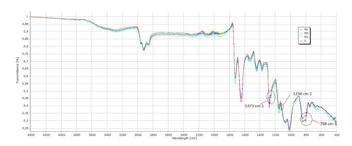
Figure 5. ATR-FTIR result of melamine applied leathers
