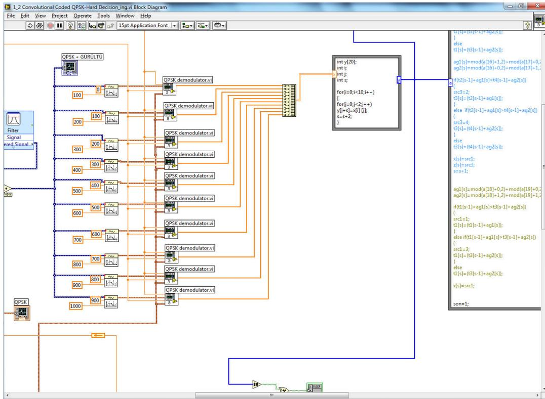
Figure10. LabVIEW Block Diagram of Receiver Side for Error Performance Analysis Experiment
