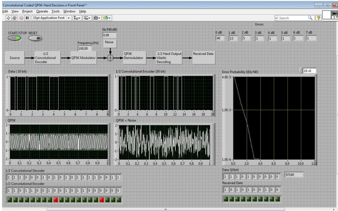
Figure11. Error Performance Experiments Front Panel
