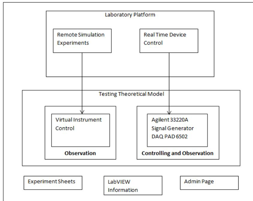
Figure12. The Block Diagram of Remotely Accessible and Controllable Laboratory Platform
