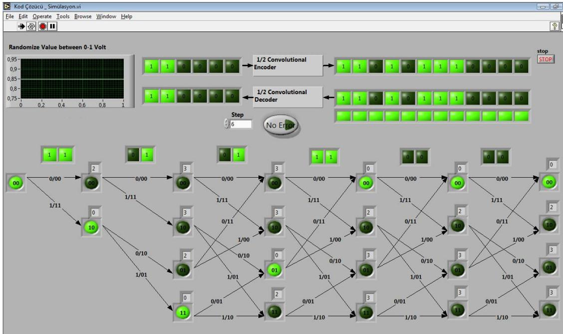
Figure8. (2,1,2) Viterbi Decoding Algorithm Experiment Front Panel
