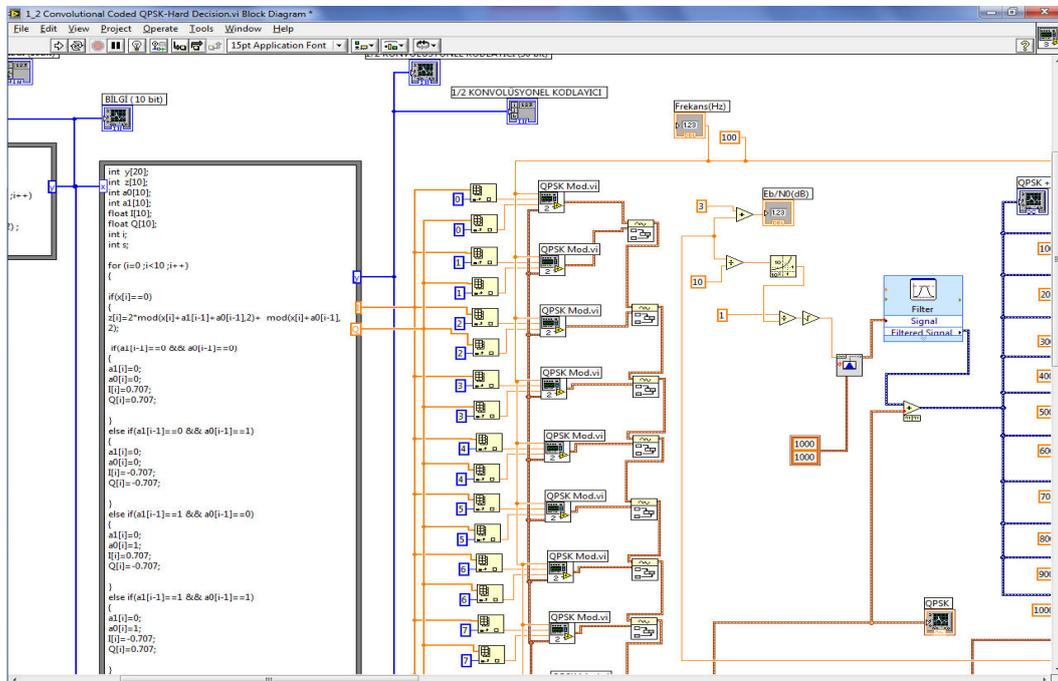
Figure9. LabVIEW Block Diagram of Transmitter Side for Error Performance Analysis Experiment
