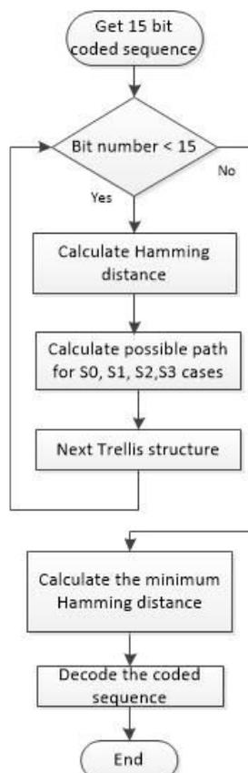
Figure 7. The flow chart of the Viterbi decoding algorithm experiment for (3,2,2) convolutional codes
