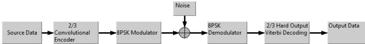
Figure1. Block diagram of Communication Systems Model
