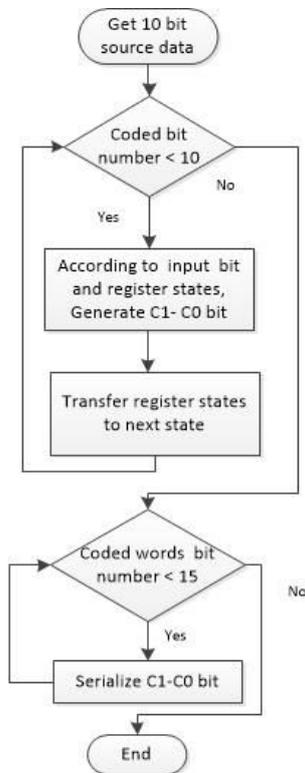
Figure 4. Flowchart of the (3,2,2) Convolutional Codes Experiment
