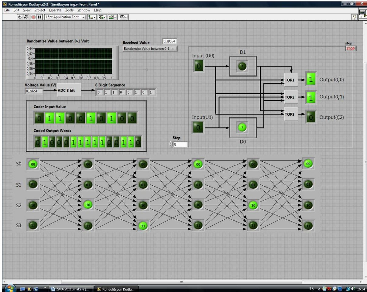
Figure5.  $(3,2,2)$  Convolutional Codes Experiment Front Panel
