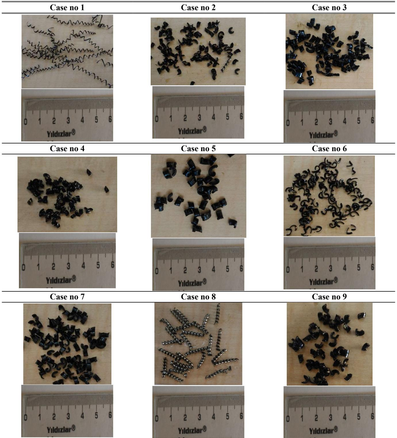
Figure 3. Photographs of chip formation from experiments
