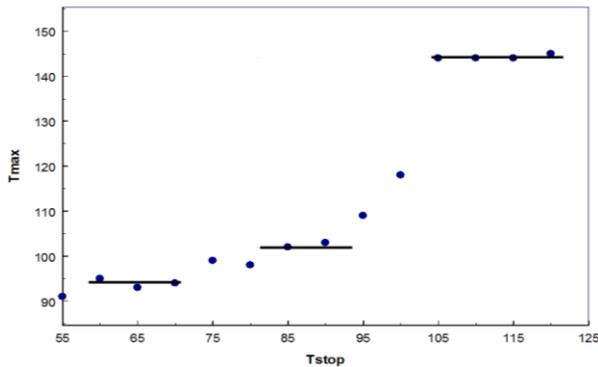
**Figure 7** Locations of possible individual peaks reached by the  $T_{max}$ - $T_{stop}$  method.
