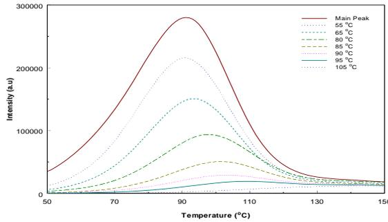
**Figure 6** The glow curves of NaCl for different  $T_{stop}$  values.
