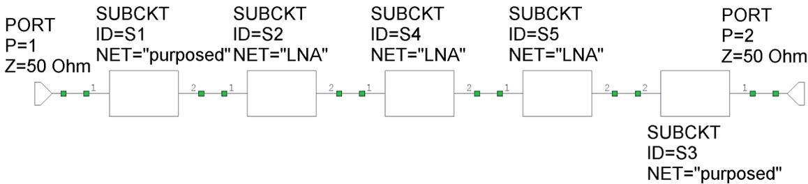
Figure 9. The circuit of three cascaded LNA application circuits with purposed BPFs.
