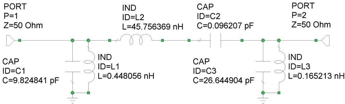
Figure 1. Purposed BPF circuit with element values.
