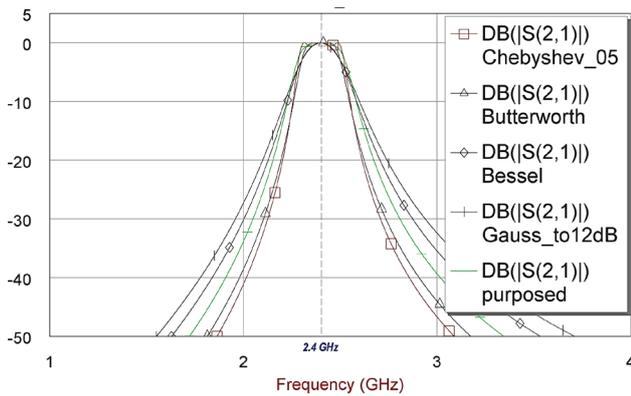
Figure 5.  $S_{21}$  graph of 5 different methods.
