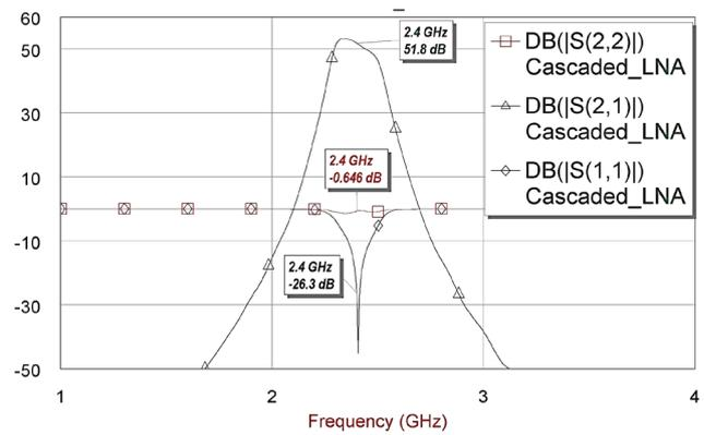
Figure 10. S parameters of cascaded system.
