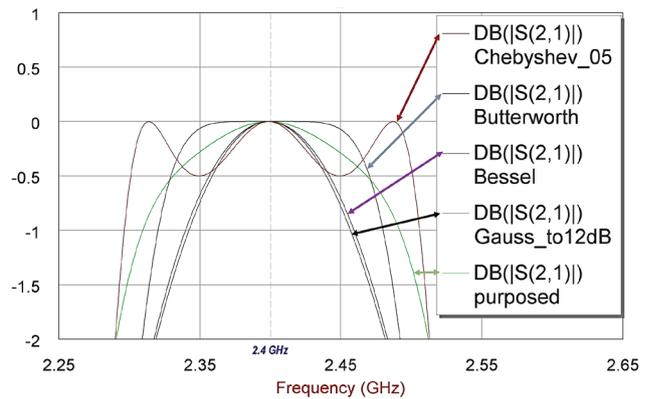
Figure 6. A close-up  $S_{21}$  graph of 5 different methods, (pass band region of Figure 5).
