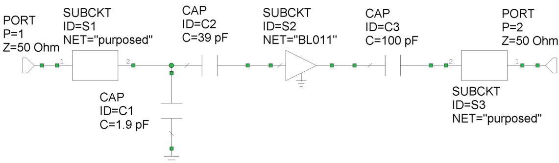
Figure 7. LNA application circuit with purposed BPFs.
