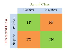
FIGURE 3. General elements of a confusion matrix in binary classification.
