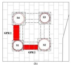
**Figure 15.** The indication of the GPR scanning regions on the lintels (each region is shown by the red color)
