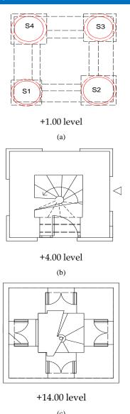
Figure 4. Plans of Four-Legged Minaret at: (a) +1.00, (b) +4.00, and (c) +14 levels
