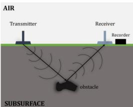
Figure 6. Schematical demonstration of the working principle of a typical GPR system
