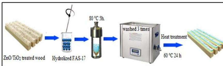
Figure 3. Schematic representation of the hydrophobization
