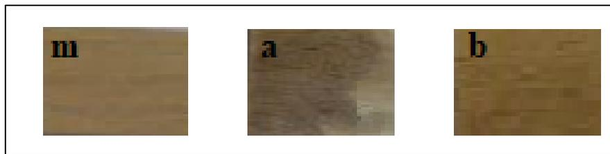
Figure 9. The color parameters of massive wood (m), ZnO/TiO<sub>2</sub> treated-wood (a), and ZnO/TiO<sub>2</sub>@FAS-17-treated wood (b)
