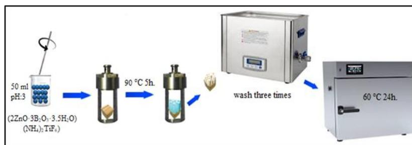
Figure 2. Schematic illustration for the synthesis of the ZnO and TiO<sub>2</sub> nanoparticles on the wood surface using a hydrothermal treatment
