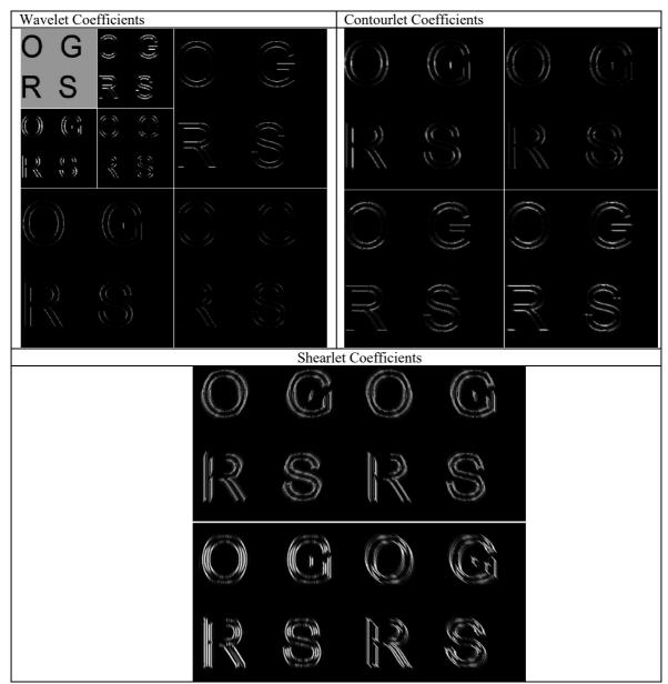
Figure 1. Wavelet, Contourlet and Shearlet Coefficients illustrations for letters O, G, R and S.
