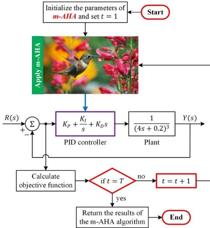
**Fig. 3.** Block diagram of m-AHA optimizer-based PID parameter estimation for liquid level system
