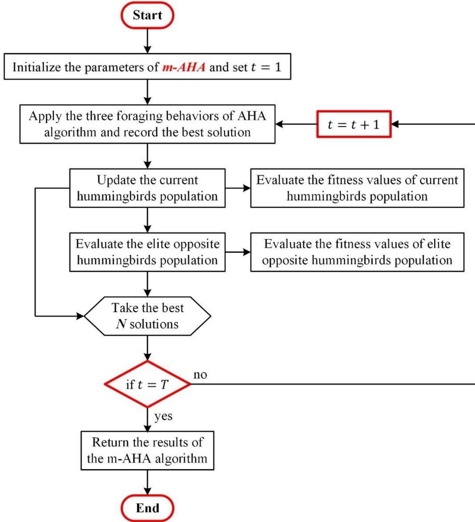
**Fig. 2.** Flowchart of recommended m-AHA optimizer
