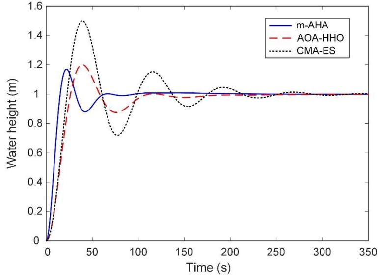
**Fig. 4.** Step response of different optimizers-based controller designs for water height
