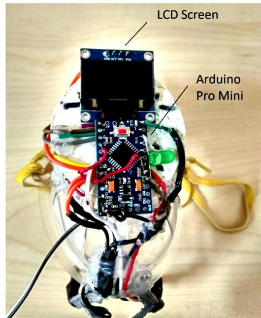
Figure 3. Replacements of Arduino Pro Mini and LCD Screen
