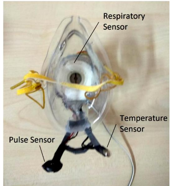
Figure 2. Replacements of electronic sensors
