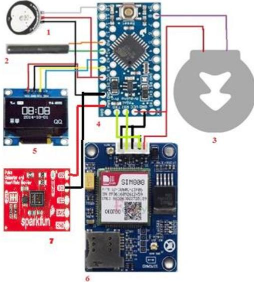
Figure 1. Circuit Design of M-Vital
