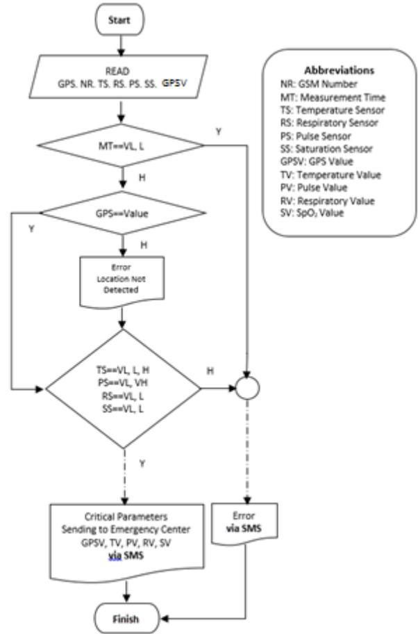
Figure 5. A part of Flowchart for M-Vital operation
