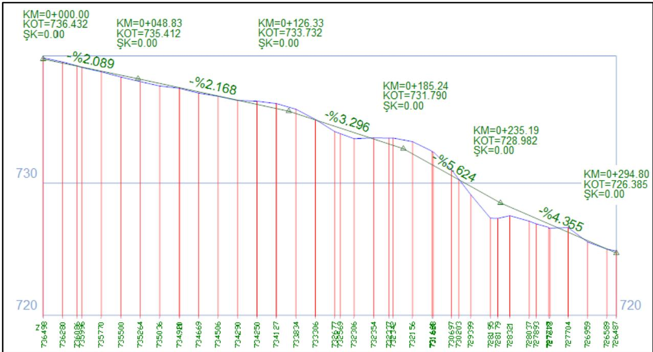
Figure 8. Horizontal profile and vertical curve definitions
