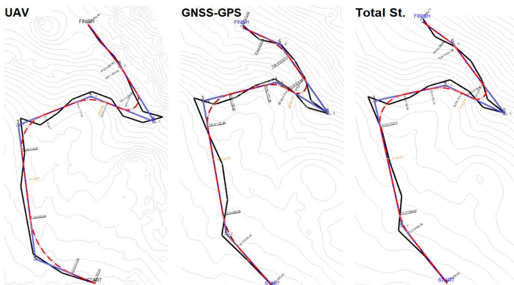
Figure 11. Preliminary alignment, road alignment and curve location determined by UAV (left), GNSS-GPS (middle), and Total Station (right) methods
