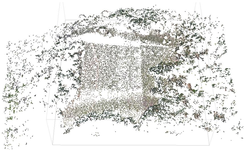
Figure 3. Tie points collected during UAV flight
