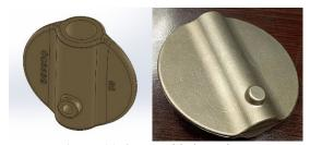
Figure 11. 3D moulded specimen
