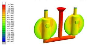
Figure 7. Casting simulation.
