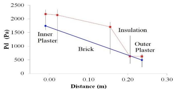
Figure 3. Internal condensation analysis for Wall 1 at 0°C,  $\phi_{in} = \phi_{out} = 0.8$
