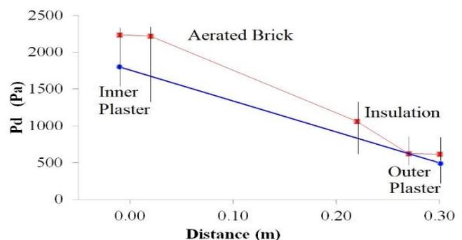
Figure 5. Internal condensation analysis for Wall 3 at 0°C,  $\phi_{in} = \phi_{out} = 0.8$
