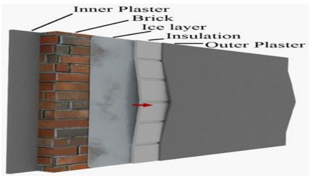
Figure 2. The ice layer that formed between layers of wall
