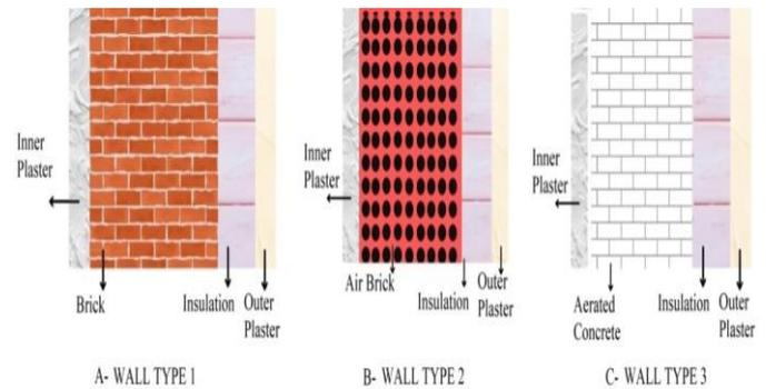
Figure 1. Wall envelope layers
