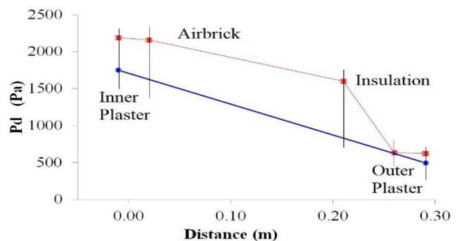
Figure 4. Internal condensation analysis for Wall 2 at 0°C,  $\phi_{in} = \phi_{out} = 0.8$
