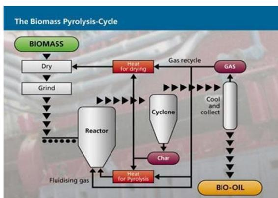
Figure 1. Pyrolysis Cycle [Abnisa and Wan Daud, 2014]
