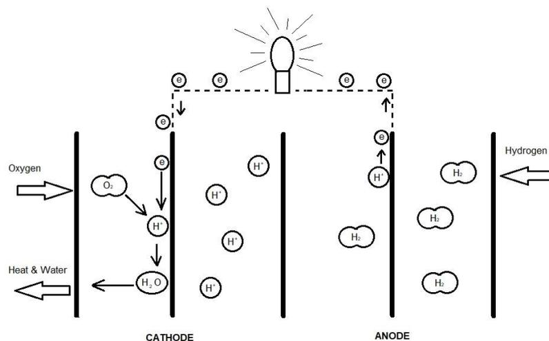
**Figure 1.** Fuel cell system proton exchange membrane working principle (U.S. Department of Energy, 2015)
