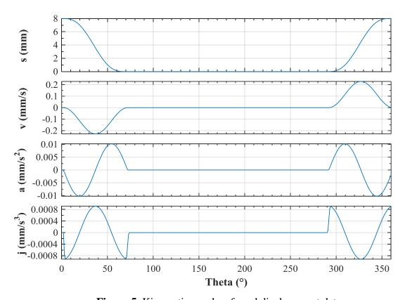
Figure 5. Kinematic graphs of used displacement data
