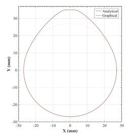
Figure 6. Overlapping of analytical and graphical approaches - flat face follower cam
