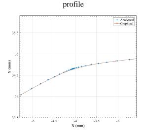
**Figure 7.** Left top region view of two profile data produced by analytical and graphical approaches - flat face follower cam profile
