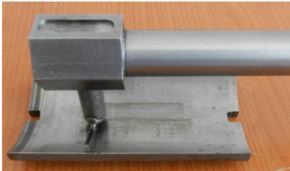
Figure 2. View of the piston ring and cylinder test specimens (used)
