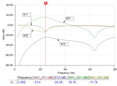
Figure 4. S Parameters of the LNA circuit via Infineon Designer powered by TinaCloud.
