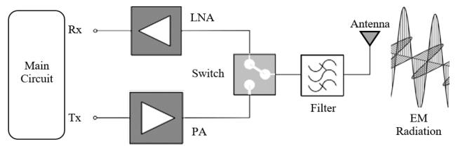
Figure 1. A basic front-end module.
