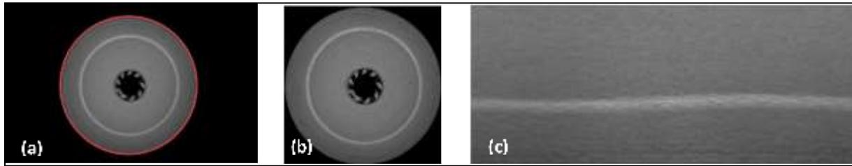
Figure 6. (a) Plotted bobbin boundary, (b) Image cropped according to bobbin outer boundary, (c) Bobbin cross-section extracted and transformed into rectangular image frame
