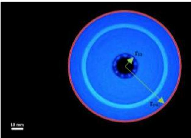
Figure 4. Bobbin diameter boundary image with Hough transformation
