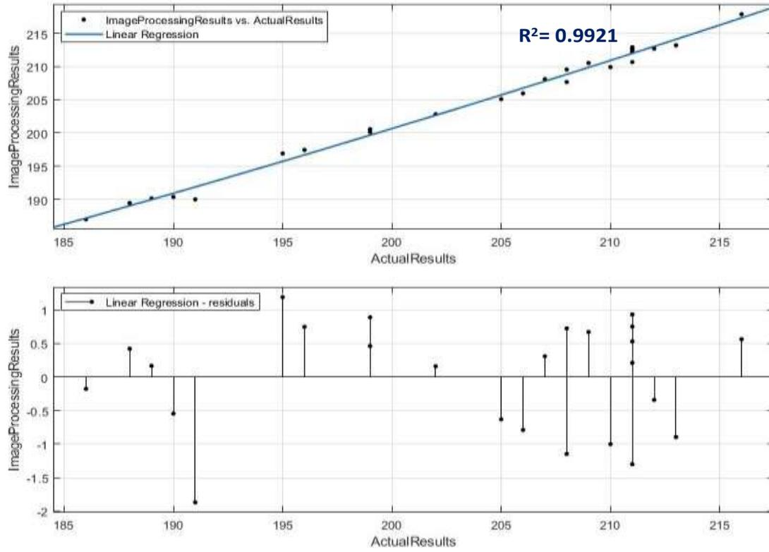
**Figure 10.** Q-Q plot of the actual and image processing measured bobbin diameter values (a) correlation graph, (b) residual graph of each measurement
