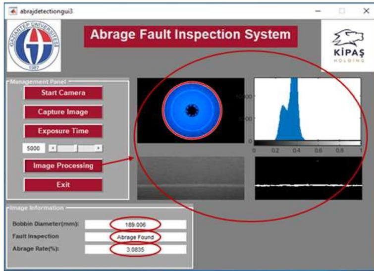
**Figure 11.** Abridge fault inspection system- User Interface
