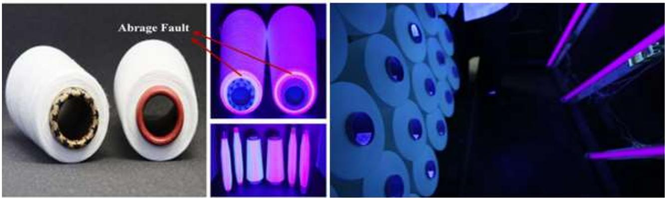
**Figure 1.** Abrage view under UV light [1, 2]
