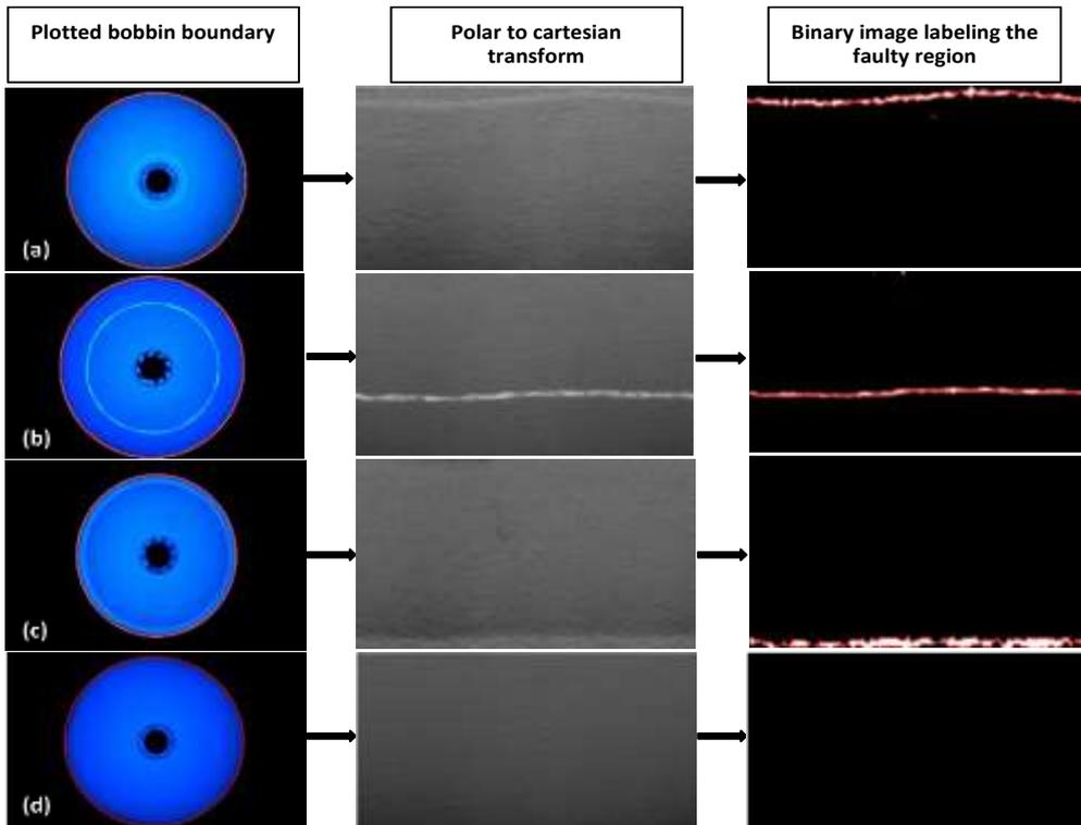
**Figure 8.** Algorithm results prepared by Local Thresholding method (a) abrage at the beginning of the bobbin, (b) abrage in the middle of the bobbin, (c) abrage at the end of the bobbin, (d) faultless bobbin
