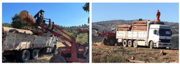
Figure 5. Hauling operation with BMC Pro 522 medium-size truck (left) and Mercedes-Benz Axor 1840 LS model large-size truck (right)
