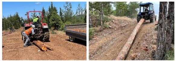
Figure 4. Skidding with Universal 445S (left) and New Holland TT55B (right) farm tractors
