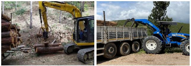
Figure 3. Loading operation with tracked loader (Sumitomo SH135) (left) and rubber-tired loader (New Holland TD 90D) (right)
