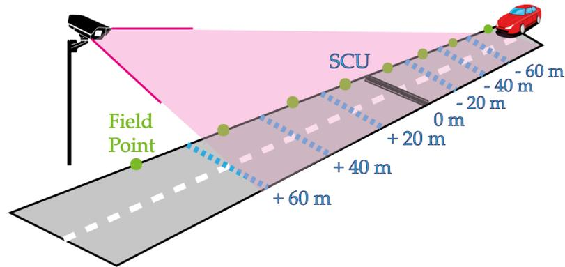
**Figure 2.** Schematic representation of distance-averaged speed measurement method.
