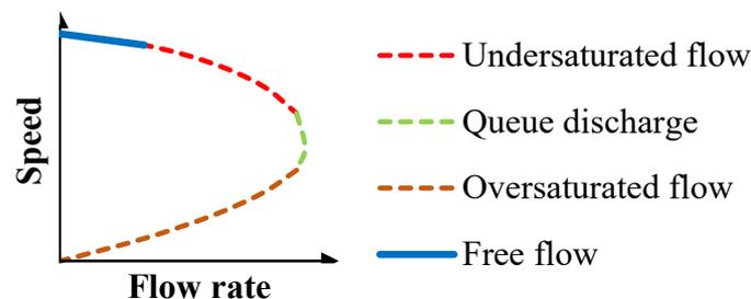
**Figure 3.** The theoretical relationship between speed and flow [24].
