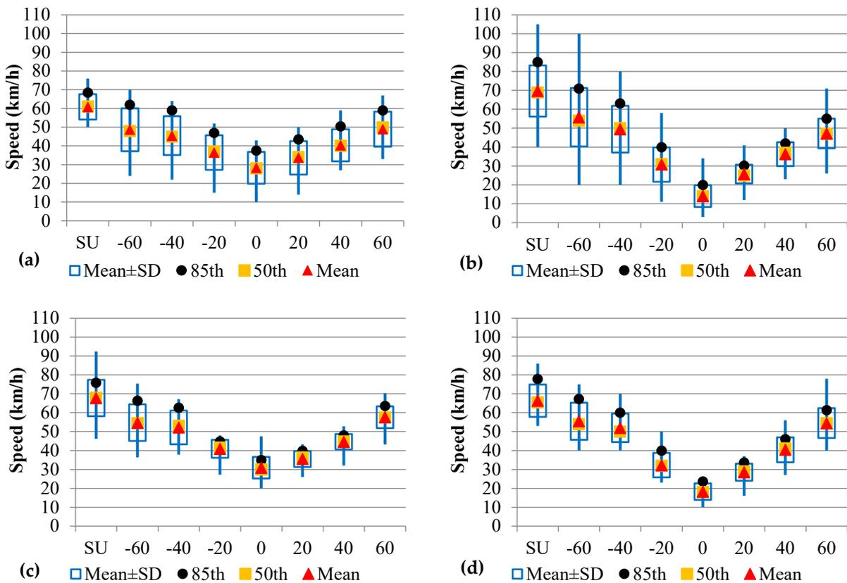
**Figure 5.** Changes of speeds measured in FF traffic regime; (a) B1 (b) B2 (c) H1 (d) H2
