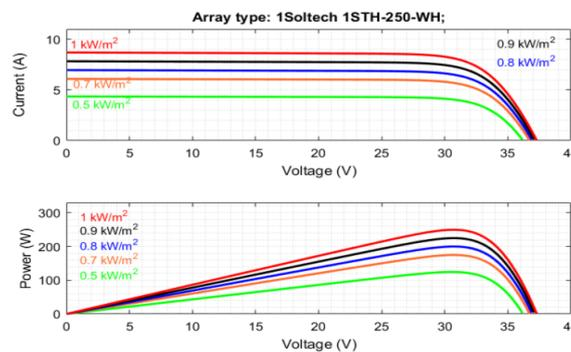
**Figure 3.** I-V and P-V curves of the PV system; at a constant  $25^\circ\text{C}$
