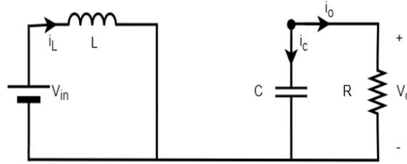
**Figure 6.** Situation when the switching element is closed
