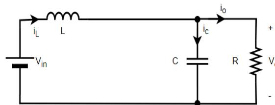
**Figure 7.** Situation when the switching element is open
