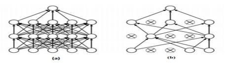
Figure 2. Dropout process
