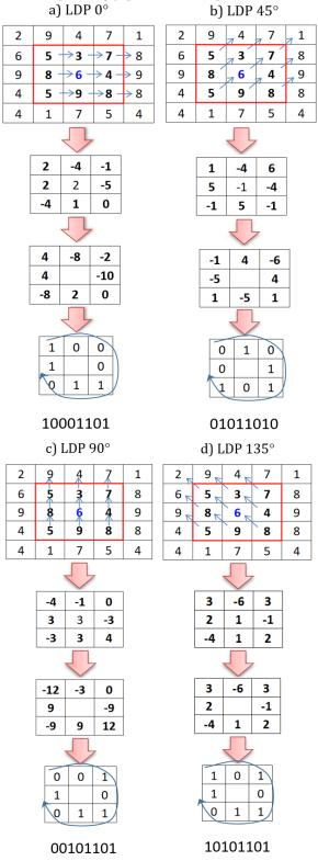
Figure 2. Example computations for first order LDP where  $\alpha$ =0°,  $\alpha$ =45°,  $\alpha$ =90° and  $\alpha$ =135°.
