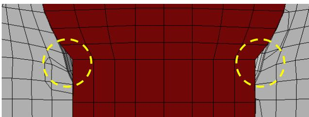
Figure 11. Gap formation at 4.5 mm (pull)
