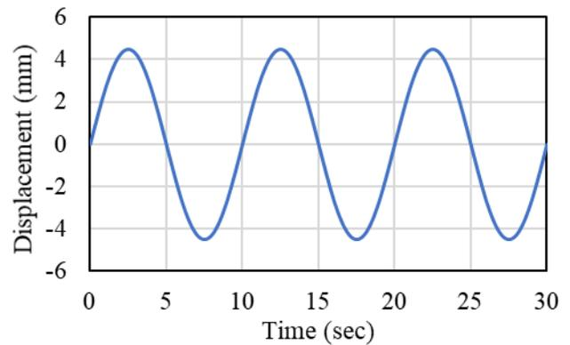
Figure 9 Applied sinusoidal displacement procedure for T-LED
