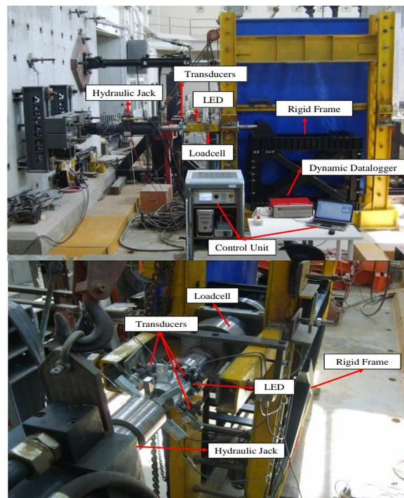
Figure 2 Dynamic tests on the developed *LED*, [13]
