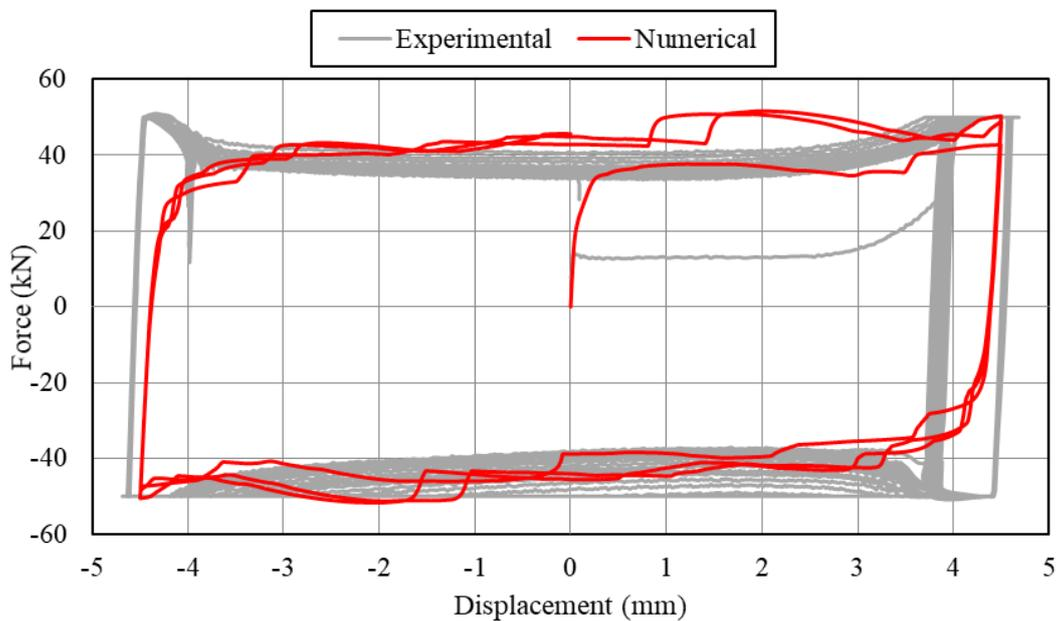
Figure 17 Comparison of experimental and numerical hysteresis of *T-LED*
