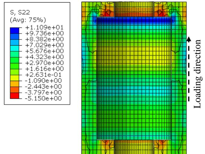
Figure 12 Stresses on the tube at 4.5 mm (pull)
