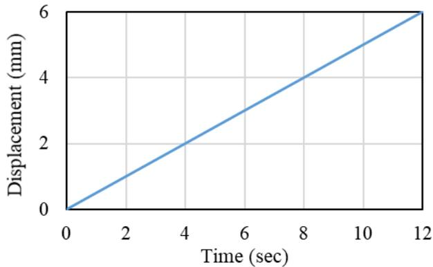
Figure 10 Ramp-type displacement procedure applied to *L-LEDs*
