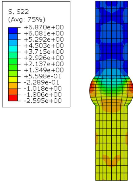
Figure 14 Stresses on the shaft at 4.5 mm (pull)
