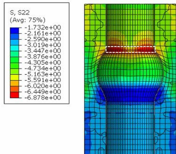
Figure 13 Stresses on the lead at 4.5 mm (pull)
