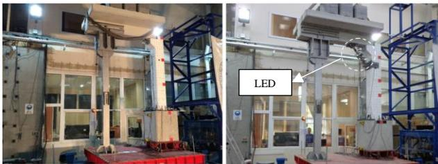
Figure 4 Precast RC beam-column connection shake table tests, [18]
