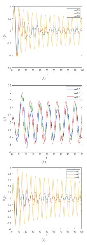
**Figure 5.** a) The inductor current, b) the CFD Capacitor current and c) the CFD Capacitor voltage vs time when the parallel circuit is fed by the sinusoidal current source simulated for three different alpha values.
