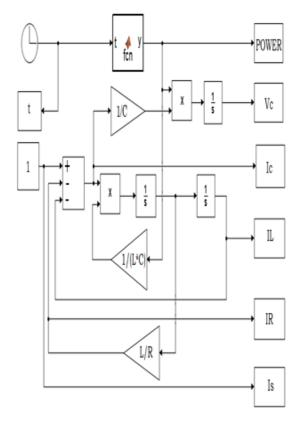
Figure 2. Simulink block diagram of the parallel circuit excited with a constant current source.
