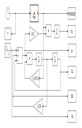
Figure 4. Simulink block diagram of the parallel circuit excited with a sinusoidal current source.
