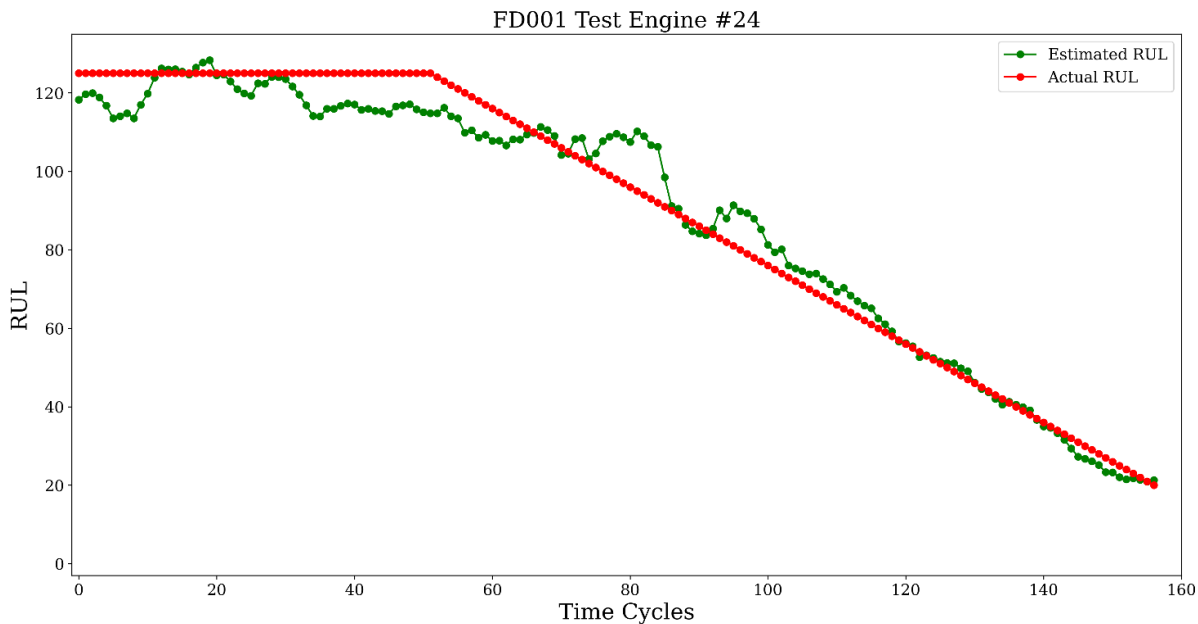
Figure 8. RUL prediction results in each time cycles engine no 24
