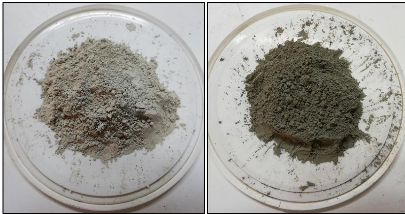
Figure 1. The appearance of BFS (left) and cement (right).
