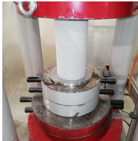
Figure 3. Compressive strength measurement of a cylindrical concrete sample.
