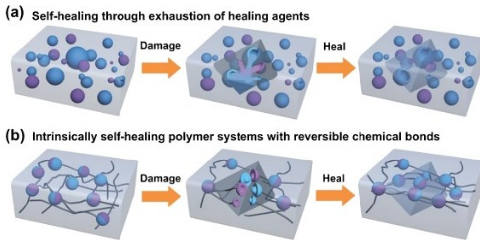
Figure 4. a) microencapsulation of healing agents and b) intrinsic self-healing mechanism [36]
