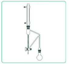
Fig. 1. System of obtained essential oil by Clevenger apparatus
