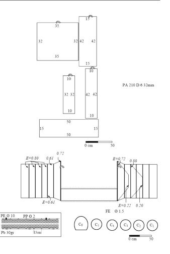
Figure 2. Technical measurements and characteristics of fyke nets (modified from Acarli, 2007)
