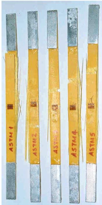
**Figure 3.** ASTM coupon - failure modes.
