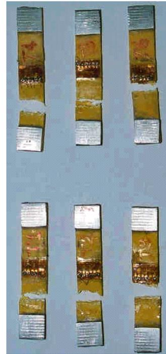
**Figure 5.** Short coupon - failure modes (transverse direction).
