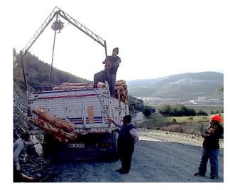
Figure 3. Electric powered winch loading
