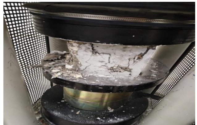
Figure 15: Standard concrete compressive test.
