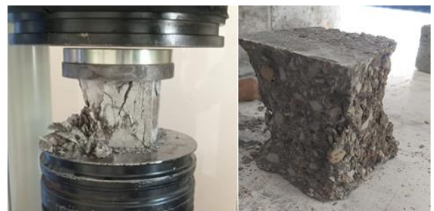
Figure 8: Compression test during and after the experiment on the specimen.
