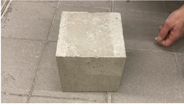
Figure 5: 15x15x15 cm cube specimen sample
