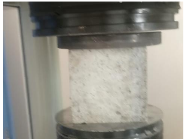
Figure 7: Compression test preparation stage of the specimen
