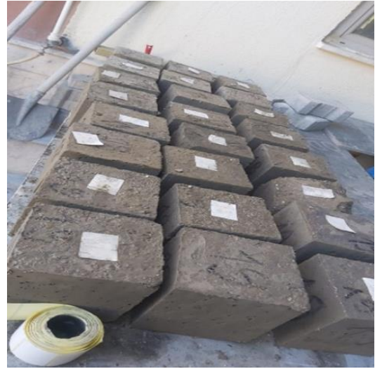
Figure 4: Specimens removed from the mold after a certain waiting period.
