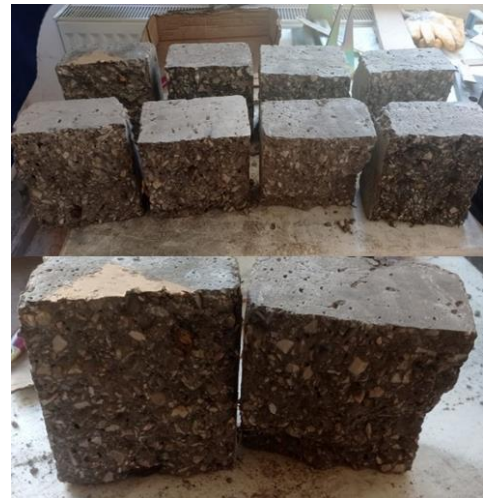
Figure 14: Final condition of specimens after the splitting tensile strength test.
