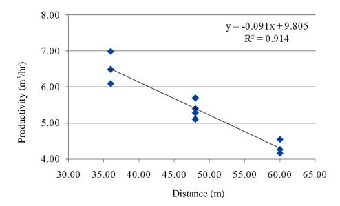
Figure 4. The relation between productivity and length of the chute system
