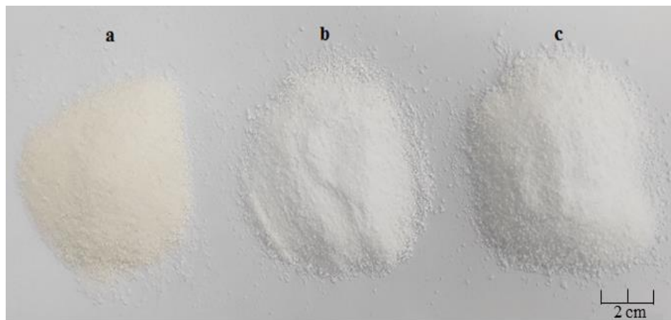
Figure 2: Additives employed in the study included: (a) SBS polymer (b) 701 polymer (c) 611 polymer
