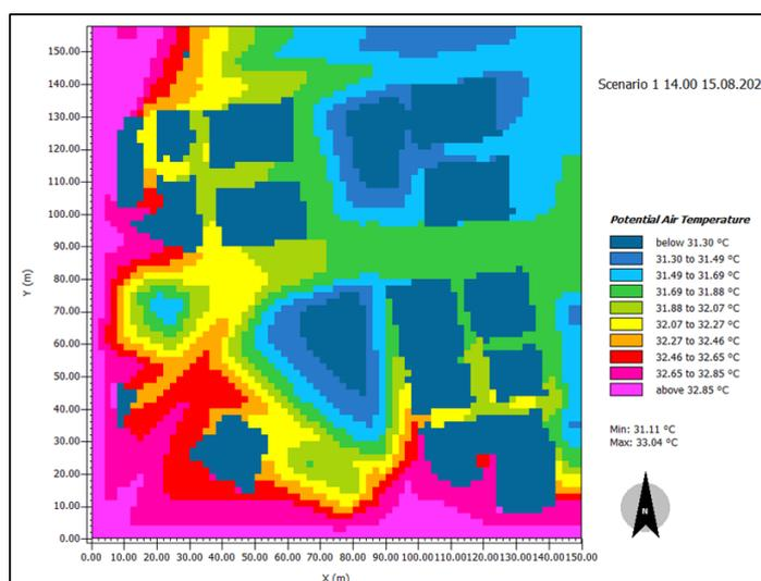
Fig. 5: Temperature Variation in the Scenario Scope
