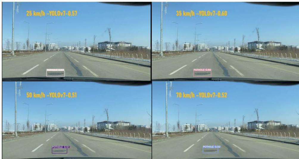
**Figure 6.** Detection performance of YOLOv7 on the same road and pothole at 25-35-50-70 km/h
