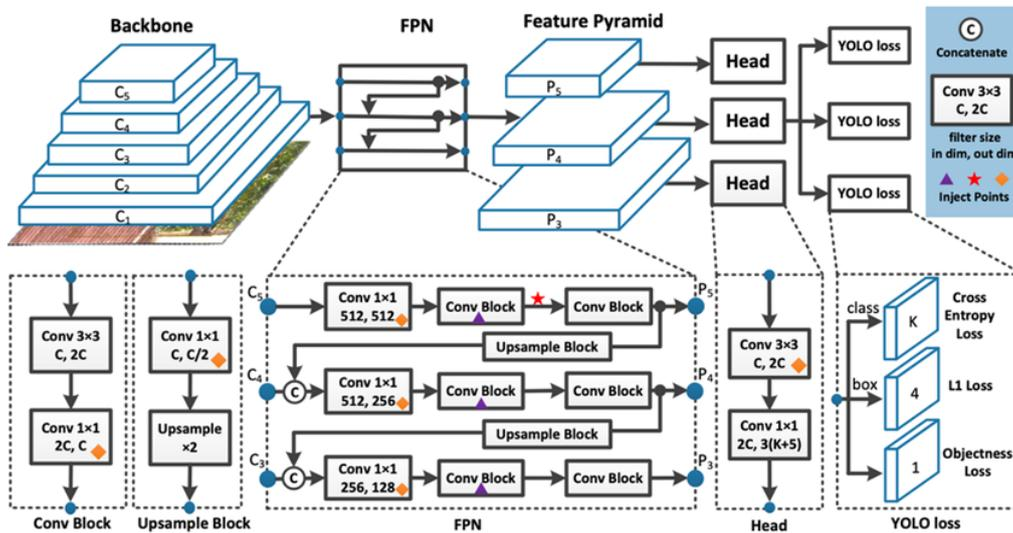
Figure 2. YOLOv7 network architecture (Wang et al, 2022)
