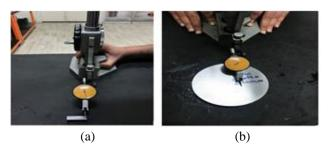
**Figure 6.** (a) Surface roughness device, (b) Sample skew check
