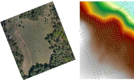
Figure 6. Total Station points (left) and Total Station based DEM (right)
