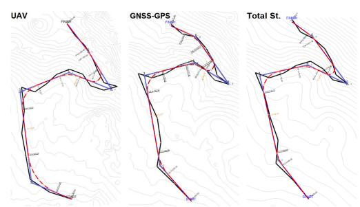
Figure 11. Preliminary alignment, road alignment and curve location determined by UAV (left), GNSS-GPS (middle), and Total Station (right) methods
