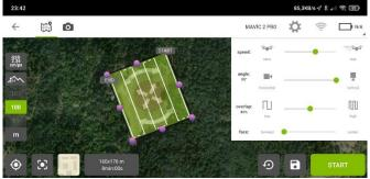
Figure 2. Pix4d flight settings
