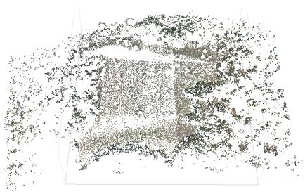
Figure 3. Tie points collected during UAV flight
