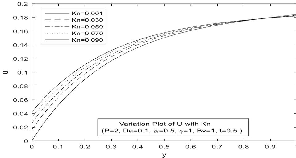
Fig. 4. Variation of Knudsen number (Kn) when the flow is induced by pressure gradient.
