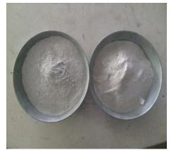
Figure 2. Passing and retaining waste glass through a No. 325 sieve
