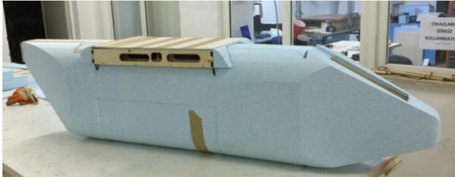
Figure 12. Covering the fuselage with foam
