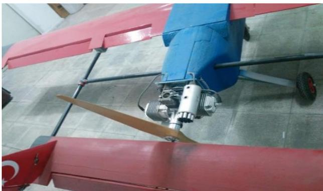
Figure 14. UAV engine mount
