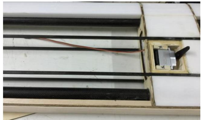
**Figure 10.** Adding servo motor to the wing
