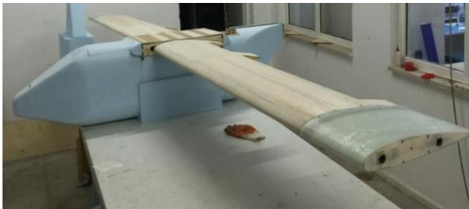
Figure 13. Wing - Body Assembly
