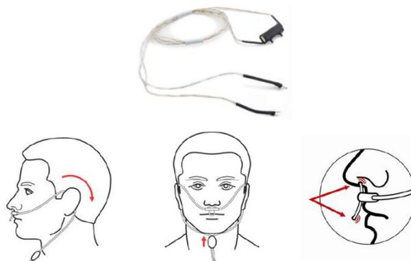
Figure 3. Airflow sensor [29]
