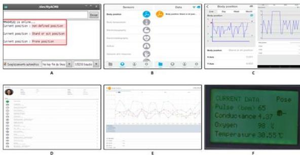
**Figure 25.** Body position results: (a) in serial monitor; (b) in the mobile application; (c) waves in the mobile application; (d) in web server; (e) waves in web server; (f) in GLCD
