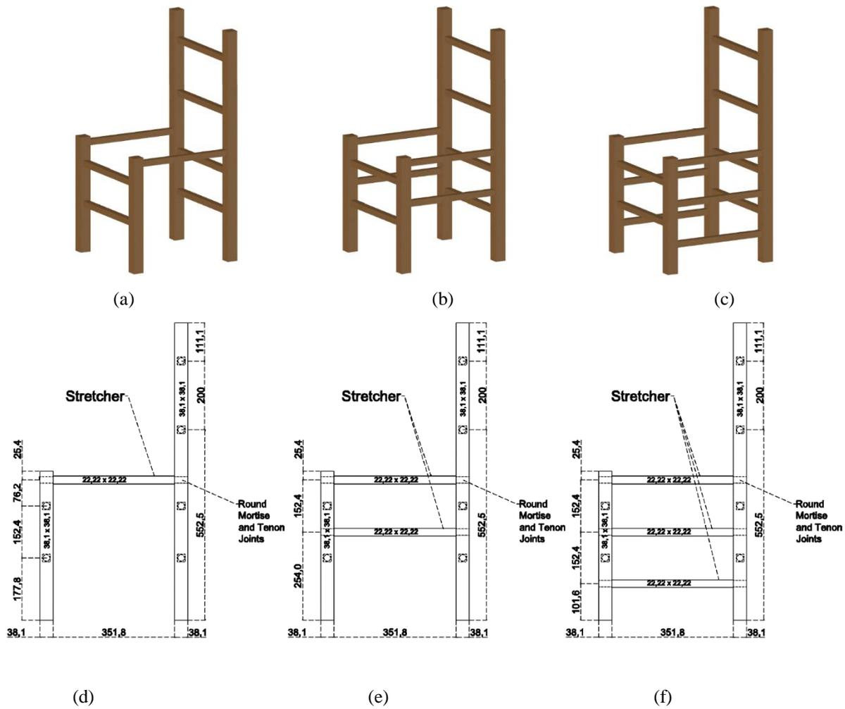
**Figure 2.** Configuration of the full-frame chair with a. one stretcher, b. two stretchers, and c. three stretchers, and dimensions and position of joints on side chair with d. one stretcher, e. two stretchers, and f. three stretchers
