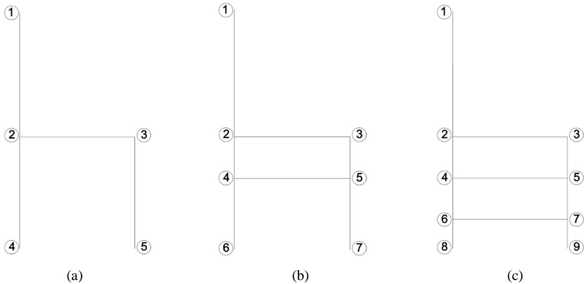
Figure 6. Nodes on chair frame for stiffness method
