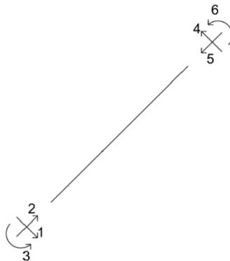
**Figure 4.** Degrees of freedom for element stiffness
