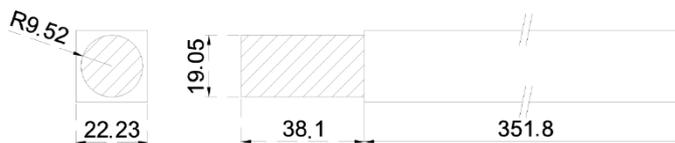
**Figure 1.** Configuration of the round mortise and tenon joints
