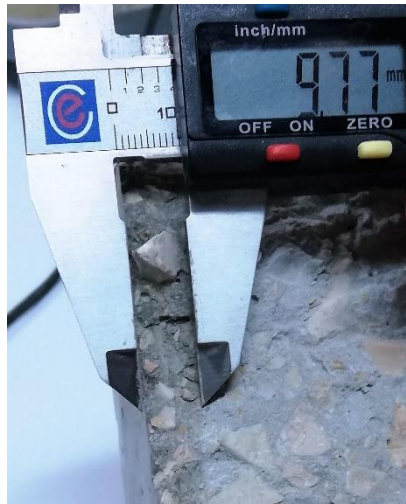
Figure 7. The process of measuring the depth of water penetration.
