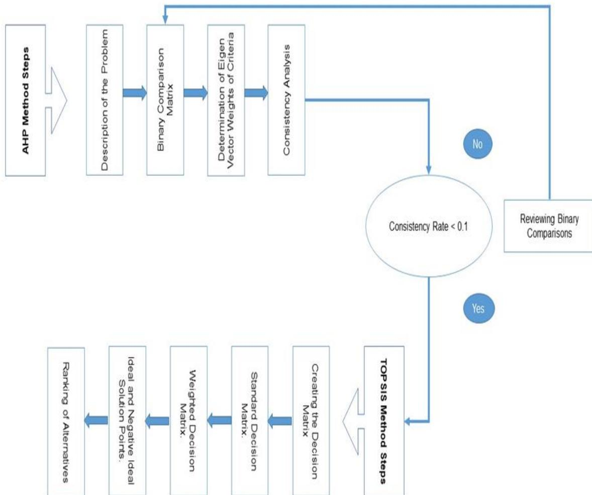
**Figure 2.** Application flow chart of AHP and TOPSIS methods.
