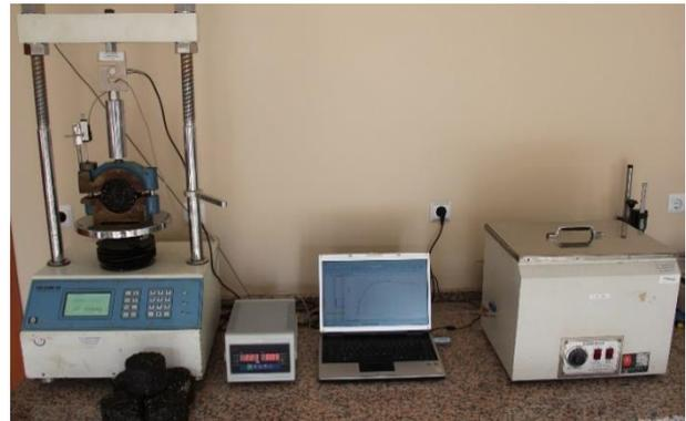
**Figure 2.** VJ Tech - TRISCAN 50 loading device
