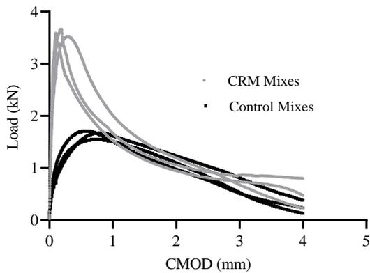
Figure 7. The work of fracture plots
