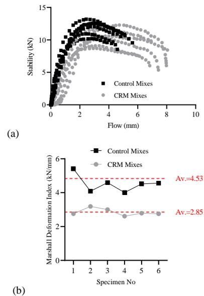
Figure 6. Marshall deformation index in specimens
