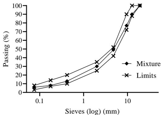
**Figure 1.** Gradation limits for HMA
