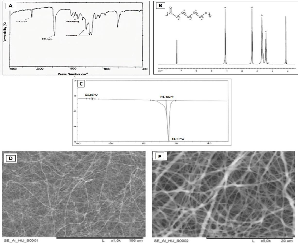
**Figure 2.** (A) FTIR spectra of  $\epsilon$ -PCL scaffolds at approximately 40.000 to 400  $\text{cm}^{-1}$  indicated by black lines, (B)  $^1\text{H-NMR}$  spectrum of  $\epsilon$ -PCL, (C) DSC thermogram of  $\epsilon$ -PCL, SEM images of micropores and macro channels of  $\epsilon$ -PCL (D; X1000), (E; X5000)
